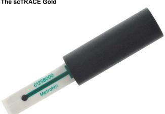
The scTRACE Gold sensor holds all three electrodes required for a voltammetric determination. Together with the electrode shaft it makes a complete electrode system which can be used in any Metrohm voltammetric measuring stand. No further electrodes are required. The working electrode is a gold microwire. Reference and auxiliary electrode, on the rear side of the sensor are screen printed electrodes.
