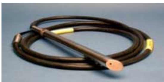
Fig. 4. A novel probe employing an angled sample interface
