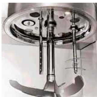
Fig. 3. The standard Bohle temperature probe was replaced with the angled NIR probe for this study
