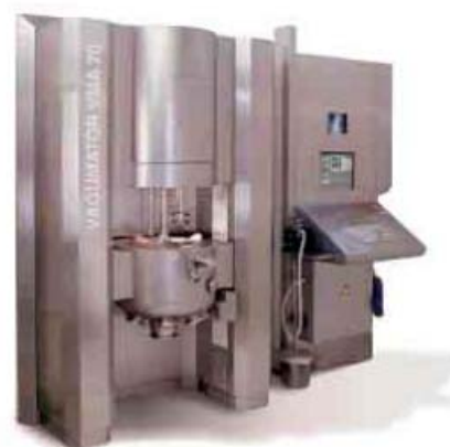
Fig. 2. Bohle single-pot high shear granulator used in study
